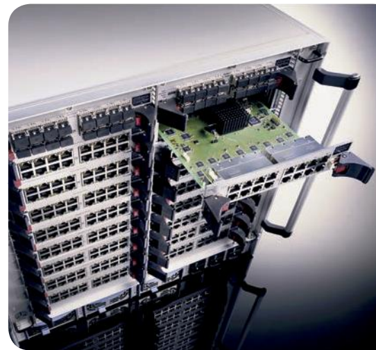
G&D CCD 288 frame with up to 288 dynamic ports to connect either CPUs or CON modules, mix of Fiber and CAT-x ports.
