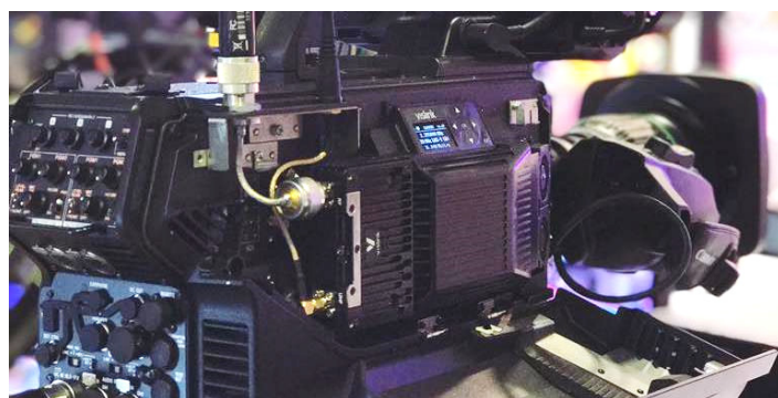
Vislink's INCAM-HS integrated into the side-panel of the Sony HDC-5500 system camera
